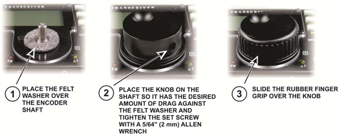
Figure 20. Mounting the VFO Knob.
