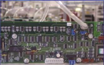
**6231A is a 4 gas analyser bench** HC - Hydrocarbon, (n-Hexane), CO<sub>2</sub> Carbon Dioxide CO Carbon Monoxide and O<sub>2</sub> Oxygen
