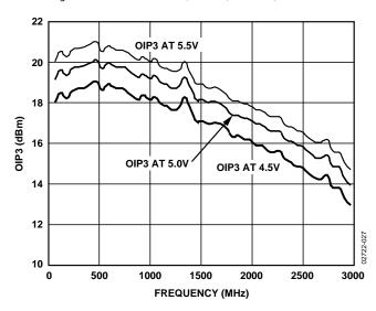
Figure 28. OIP3 vs. Frequency,  $V_S = 4.5$  V, 5 V, and 5.5 V,  $T_A = 25$  °C
