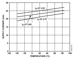
Figure 19. Supply Current vs. Temperature,  $V_S = 2.7 \text{ V}$ , 3 V, and 3.3 V
