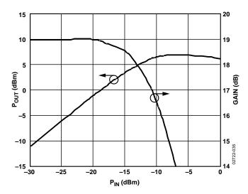
Figure 36. Output Power and Gain vs. Input Power,  $V_S = 5 V$ ,  $T_A = 25$ °C, f = 900 MHz
