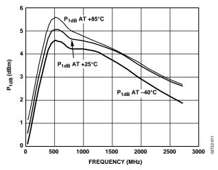
Figure 12.  $P_{1dB}$  vs. Frequency,  $V_S = 3$  V,  $T_A = -40$ °C, +25°C, and +85°C
