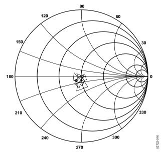
Figure 17.  $S_{11}$  vs. Frequency,  $V_S = 5$  V,  $T_A = 25$ °C, 100 MHz  $\leq f \leq 3$  GHz
