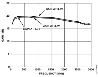
Figure 4. Gain vs. Frequency,  $V_S = 2.7 \text{ V}$ , 3 V, and 3.3 V,  $T_A = 25 ^{\circ}\text{C}$
