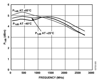
Figure 26.  $P_{1dB}$  vs. Frequency,  $V_S = 5 V$ ,  $T_A = -40 ^{\circ}\text{C}$ ,  $+25 ^{\circ}\text{C}$ , and  $+85 ^{\circ}\text{C}$
