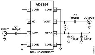
Figure 40. Evaluation Board Schematic
