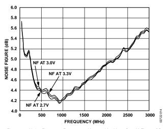
Figure 15. Noise Figure vs. Frequency,  $V_S = 2.7 \text{ V}$ , 3 V, and 3.3 V,  $T_A = 25 ^{\circ}\text{C}$
