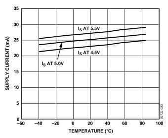
Figure 34. Supply Current vs. Temperature,  $V_S = 4.5 \text{ V}$ , 5 V, and 5.5 V
