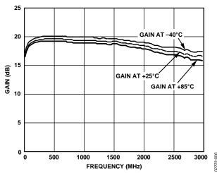
Figure 7. Gain vs. Frequency,  $V_S = 3 V$ ,  $T_A = -40 ^{\circ}C$ ,  $+25 ^{\circ}C$ , and  $+85 ^{\circ}C$
