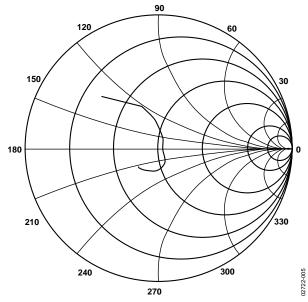
Figure 6.  $S_{22}$  vs. Frequency,  $V_S = 3 V$ ,  $T_A = 25 ^{\circ}$ C,  $100 \text{ MHz} \le f \le 3 \text{ GHz}$
