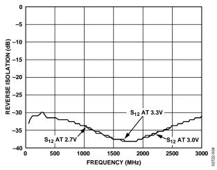
Figure 5. Reverse Isolation vs. Frequency,  $V_S = 2.7 \text{ V}$ , 3 V, and 3.3 V,  $T_A = 25 ^{\circ}\text{C}$
