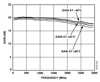
Figure 24. Gain vs. Frequency,  $V_S = 5$  V,  $T_A = -40$ °C, +25°C, and +85°C
