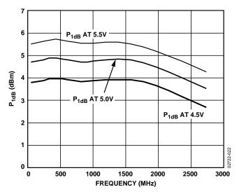
Figure 23.  $P_{1dB}$  vs. Frequency,  $V_S = 4.5 \text{ V}$ , 5 V, and 5.5 V,  $T_A = 25 ^{\circ}\text{C}$
