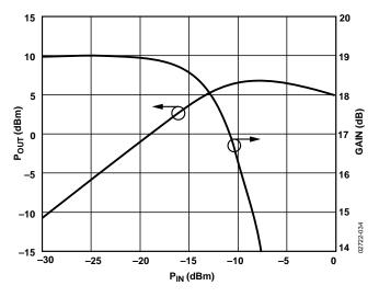
Figure 35. Output Power and Gain vs. Input Power,  $V_S = 3 V$ ,  $T_A = 25$ °C, f = 900 MHz
