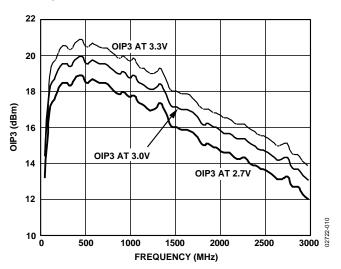
Figure 11. OIP3 vs. Frequency,  $V_S = 2.7 \text{ V}$ , 3 V, and 3.3 V,  $T_A = 25 ^{\circ}\text{C}$
