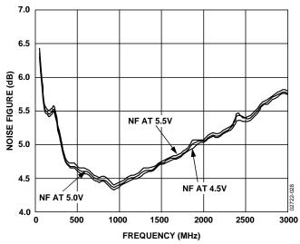
Figure 29. Noise Figure vs. Frequency,  $V_S = 4.5 \text{ V}$ , 5 V, and 5.5 V,  $T_A = 25 ^{\circ}\text{C}$
