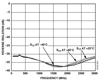
Figure 25. Reverse Isolation vs. Frequency,  $V_S = 5 V$ ,  $T_A = -40 ^{\circ}$ C,  $+25 ^{\circ}$ C, and  $+85 ^{\circ}$ C
