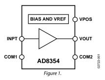
The noise figure is 4.2 dB at 900 MHz. The reverse isolation  $(S_{12})$  is -33 dB at 900 MHz.
