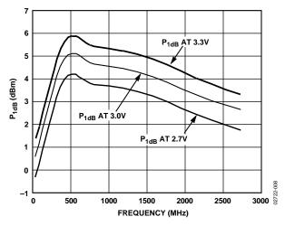
Figure 9.  $P_{1dB}$  vs. Frequency,  $V_S = 2.7 \text{ V}$ , 3 V, and 3.3 V,  $T_A = 25 ^{\circ}\text{C}$
