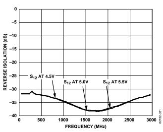
Figure 22. Reverse Isolation vs. Frequency,  $V_S$  = 4.5 V, 5 V, and 5.5 V,  $T_A$  = 25 °C
