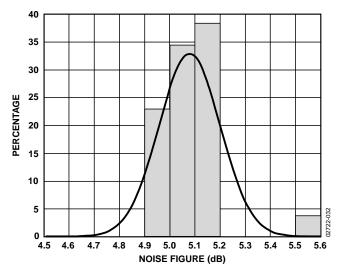
Figure 33. Distribution of Noise Figure,  $V_S = 5 \text{ V}$ ,  $T_A = 25 ^{\circ}\text{C}$ , f = 2.2 GHz
