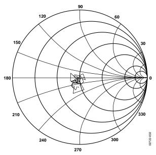
Figure 3.  $S_{11}$  vs. Frequency,  $V_S = 3$  V,  $T_A = 25$ °C, 100 MHz  $\leq f \leq 3$  GHz
