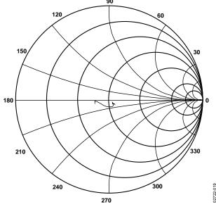
Figure 20.  $S_{22}$  vs. Frequency,  $V_5 = 5$  V,  $T_A = 25$ °C, 100 MHz  $\leq f \leq 3$  GHz
