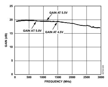
Figure 21. Gain vs. Frequency,  $V_S = 4.5 \text{ V}$ , 5 V, and 5.5 V,  $T_A = 25 ^{\circ}\text{C}$
