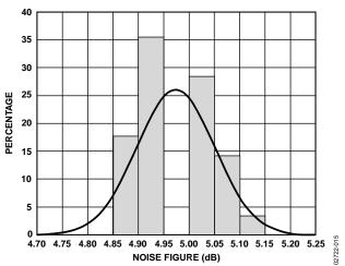
Figure 16. Distribution of Noise Figure,  $V_S = 3 \text{ V}$ ,  $T_A = 25 ^{\circ}\text{C}$ , f = 2.2 GHz
