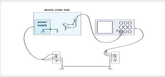
Connecting the ground lead of an oscilloscope probe to the ground in the circuit-under-test results in a ground loop if the circuit is "grounded" to earth ground.
