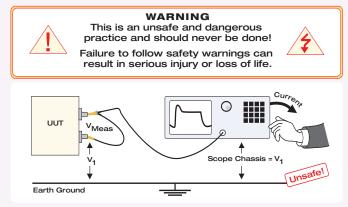
A floating measurement in which dangerous voltages occur on the oscillioscope chassis. V1 may be hunderouds of volts!
