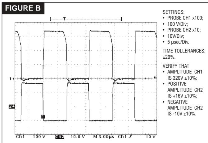
G) Repeat this test on Q2 as well using the differential probe.
