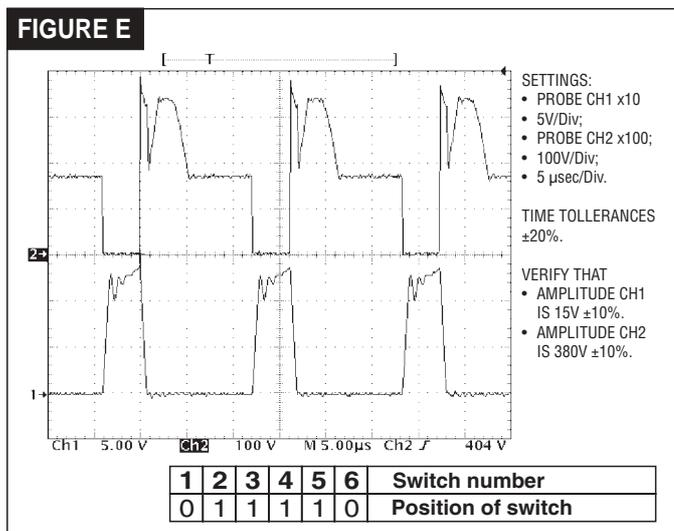
**C) Checking the secondary diode voltages:**
