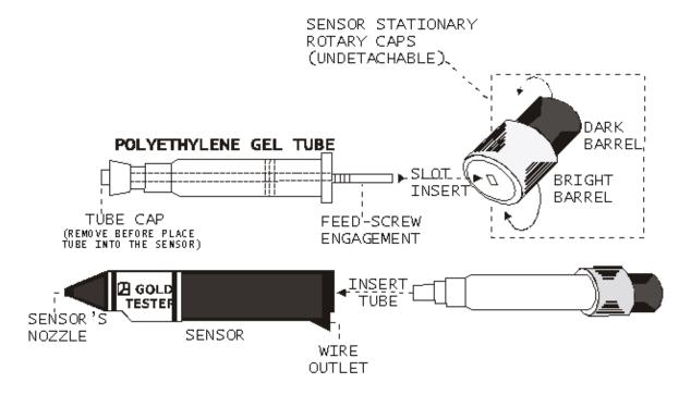
Sensor and Polyethylene Gel tube
