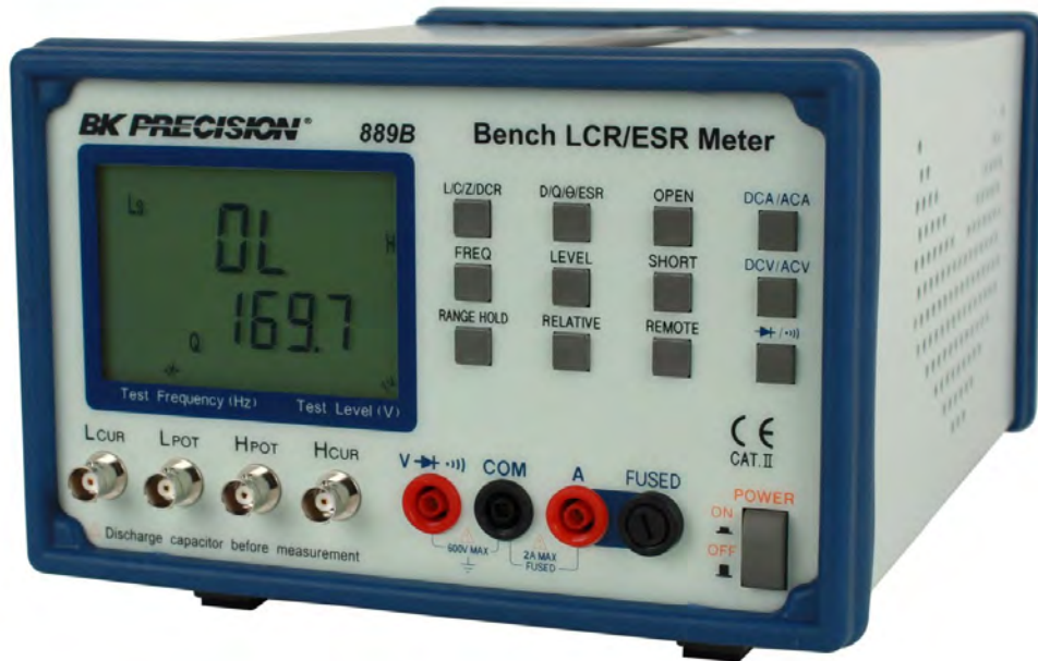
Figure 16: B&K Precision 889B bench LCR meter with voltage/current measurement capabilities
