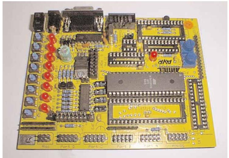
3.3V/5V operation and brownout circuitry are supported. Finally, all port pins are brought out to separate pin headers for easy expansion and signal monitoring.
